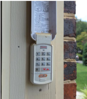
Outside door opener key pad
